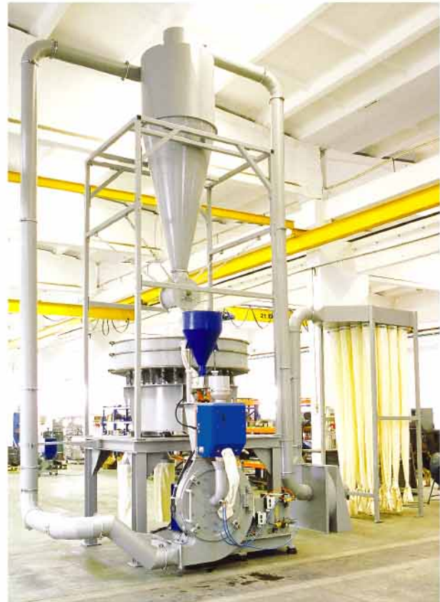
Pulverizing system including PM 500, screening machine & suction system
